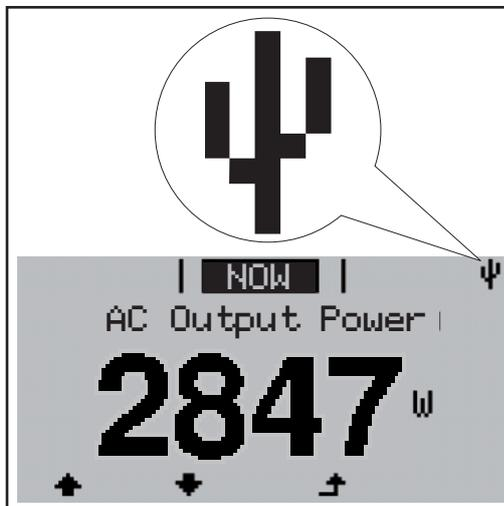
If the inverter detects a USB stick, the USB symbol will appear in the top right corner of the display.
