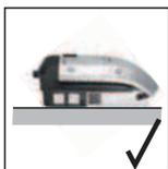
The inverter is suitable for horizontal installation.
