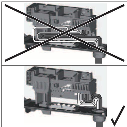
If AC cables are laid over the shaft of the DC main switch or across the connection block of the DC main switch, they may be damaged when the inverter is swung in, or they may even prevent the inverter from being swung in.
