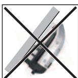
Do not install the inverter such that it overhangs with its connection sockets facing downwards.
