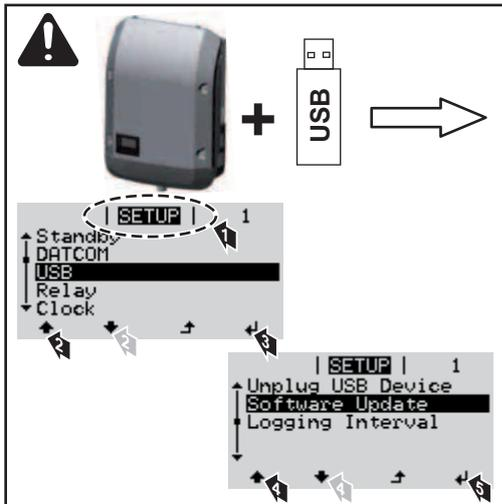
If the inverter is supplied with a USB stick, the inverter software must be updated as soon as the inverter has been commissioned:
