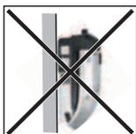
Do not install the inverter such that it overhangs with its connection sockets facing upwards.
