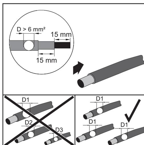
For double insulated DC connection leads with a cable diameter greater than 6 mm<sup>2</sup>, 15 mm of the outer jacket must be removed in order to connect the cable to the DC terminal.
